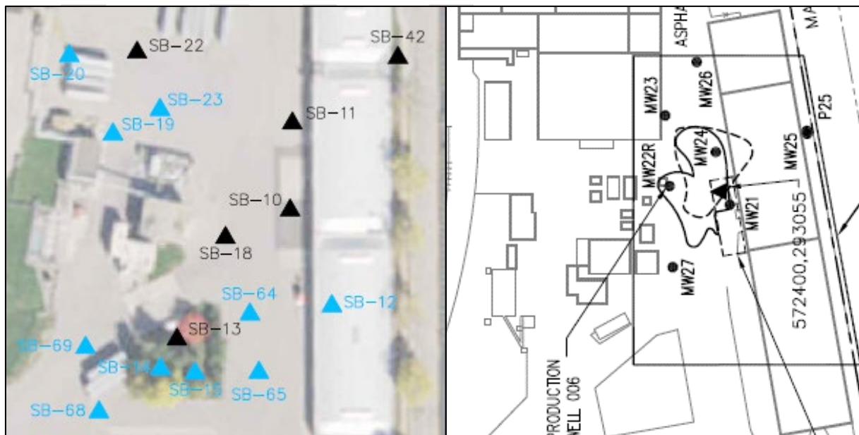
Figure 4. Closed Site #3 with 2017 data near site (left) and 1996 (right) extent of contamination.
