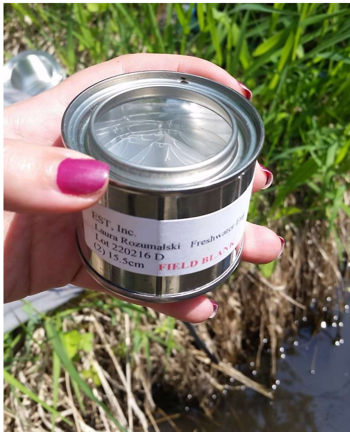
Figure 5: Field blank exposed to air at each site during deployment and retrieval
